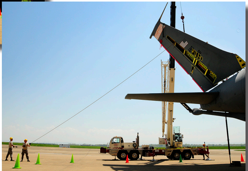
KC-135R model sits in the orange hangar awaiting maintenance (above) Members of the Repair and Reclamation Shop (right) help to sturdy the tail as the crane lifts it back into place (Air National Guard photo by Tech. Sgt. Kendra M Owenby, 134 ARW Public Affairs)
