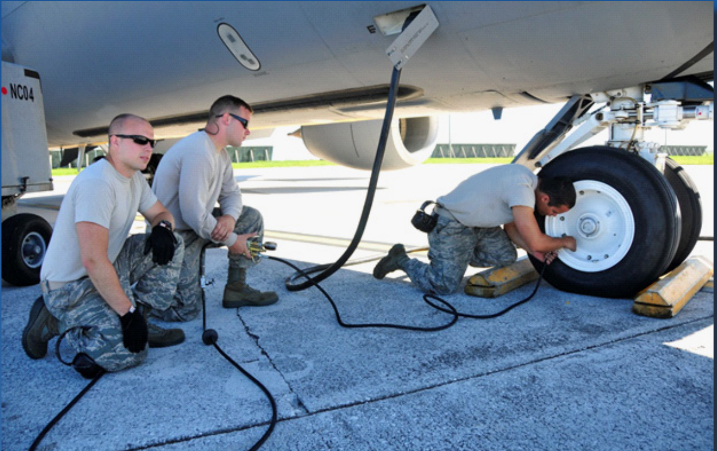
Members of the 134th Air Refueling Wing Maintenance Squadron perform tire pressure checks on a KC-135R Stratotanker during a deployment to Andersen Air Force Base, Guam (U.S. Air National Guard photo by Staff Sgt. Ben Mellon).
