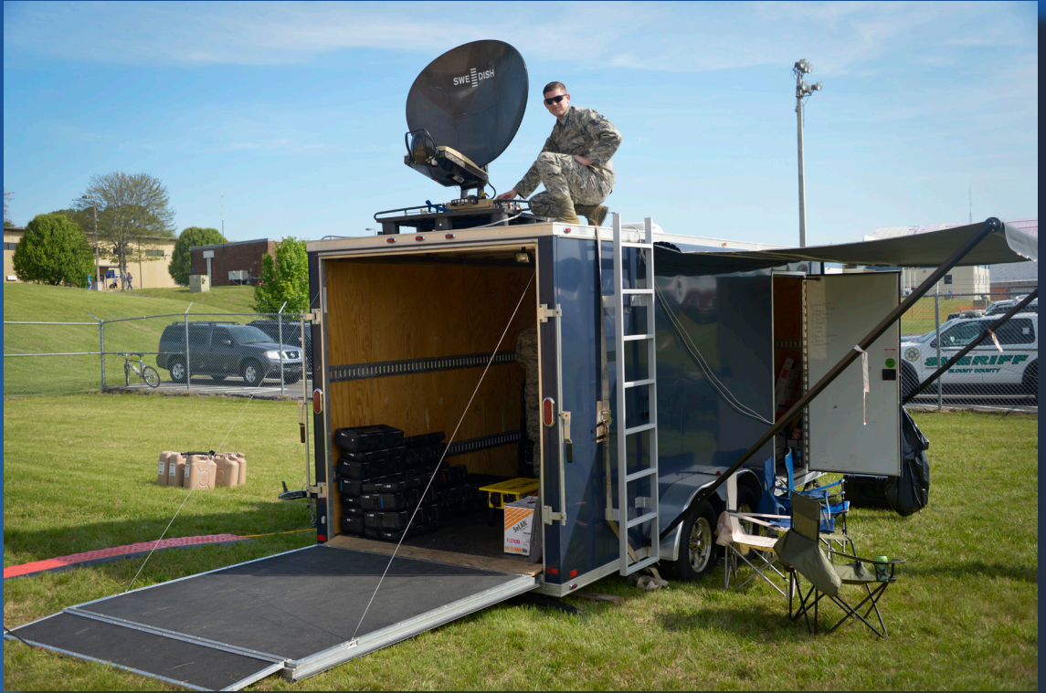
Airmen from the 119th Command and Control Squadron set up the Joint Incident Site Communication Capability Terminal (JISCC) at McGhee Tyson Air National Guard Base in preparation for the Smoky Mountain Air Show on April 16. The terminal is a system that allows different types of equipment to interface providing communication capability. (U.S. Air National Guard photos by Master Sgts. Kendra Owenby & Jon Ladue, 134 ARW Public Affairs)
